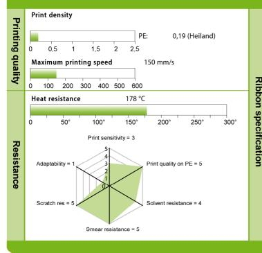
Quality level: Resin Flat-head Basefilm: PET 4,5 μm Ribbon:  $8,3 \mu m \pm 0,4 \mu m$ Colour: white Optical density 0,33 (Heiland)
