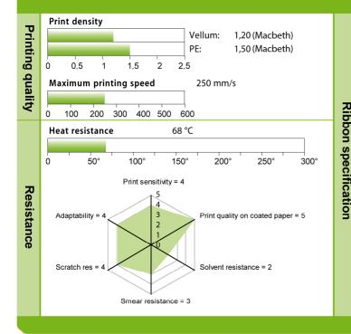
Quality level: Wax/Resin Flat-head Basefilm: PET 4,5 μm
