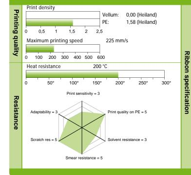
Ribbon:  $9,0 \ \mu m \pm 0,4 \ \mu m$ Colour: Process black Optical density 0,65 (Heiland) ribbon: Ink melting 83 °C point: Approvals: Halogen-free, UL approved on many label materials
