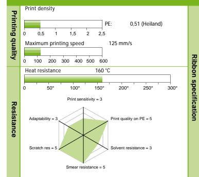
Basefilm: PET 4,5 μm Ribbon:  $6,5 \, \mu m \pm 0,5 \, \mu m$ Colour: White Optical density 0,16 (Heiland) ribbon: Ink melting 180 °C point:
