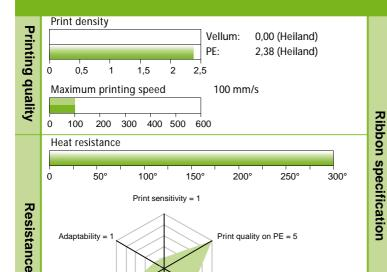
Quality level: Resin Flat-head Basefilm: PET 5,7 µm Ribbon: 7,0 µm Colour: 300 C Optical density 1,50 (Heiland) ribbon:
