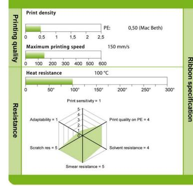
Quality level: Resin Flat-head Basefilm: PET 4,5 μm
