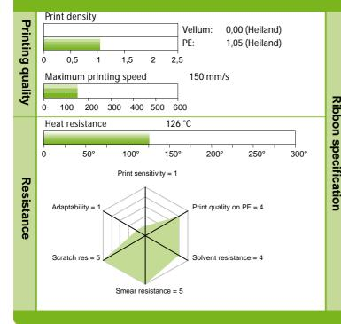
Basefilm: PET 4,5 μm Ribbon:  $5,9 \mu m \pm 1,0 \mu m$ 871 C Colour: Optical density ribbon: Ink melting 90 °C point:
