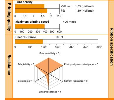
Quality level: Wax/Resin Near-edge Basefilm: PET 4,5 μm Ribbon:  $7,5~\mu m~\pm 0,5~\mu m$ Colour: **Process Black Optical density** 0,78 (Heiland) ribbon: Ink melting 80 °C point:
